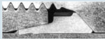
Cross section - Profile ring
