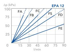
are obtained from test done at the UFI HYDRAULIC DIVISION Laboratory, according to the specification ISO 3968. In case of discrepancy, please check the contamination level, viscosity and features of the fluid in use.
